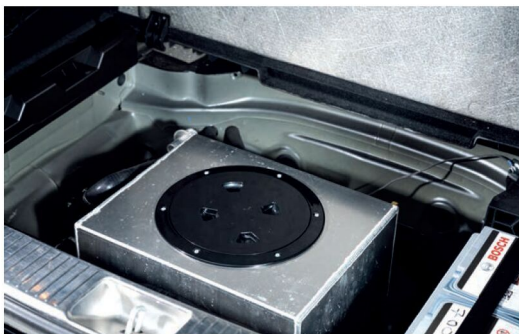
△ Icebox in boot part of this C63’s cooling system.
